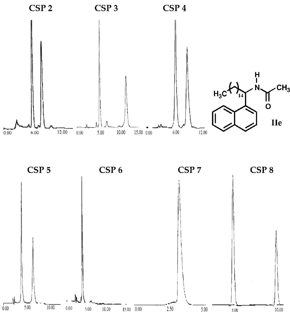
Fig. 2. Chromatographic separation of racemic *N*-acetyl-1-naphthylaminohexadecane (IIe) on CSPs 2–8 (see footnote “a” to Table 1 for chromatographic conditions).
